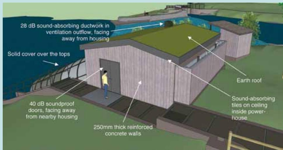
The scheme is located within the active floodplain, so the turbine is designed to withstand a 100 year flood, with the additional impact of high spring tides and potential for increased river levels due to climate change.
